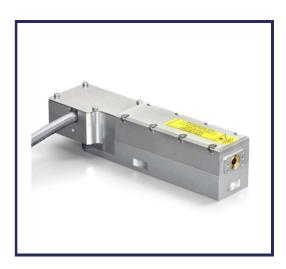
For generating high peak power Green pulses of a few hundred picoseconds, microchip lasers are economical, compact, and reliable. 532nm pulses are subsequently produced by harmonic conversion from the IR systems, the same sealed package being used for either wavelength. The SNG II series are designed for high average power, delivering multi-kW peak power at repetition rates up to 40kHz.
