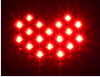
Fig. 6: Top: LED module as is used in traffic light systems Right: Examples of radiation patterns in the near field (top diagram) and the far field (bottom diagram)
